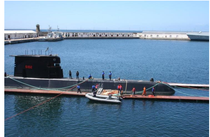
SAN submarine in deperming range
