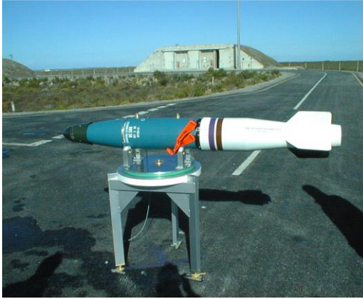
Rotating the platform on a 2D / 3D non-magnetic test jig
